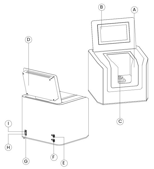
**A - Door for access to the work area.** Movable door with a transparent section that allows monitoring of ongoing operations while maintaining high safety standards.
